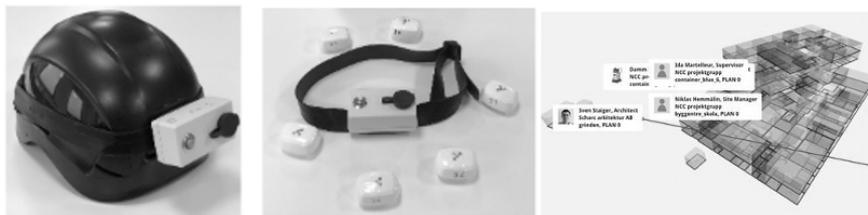
*Figure 4: The smart helmet with IoT device, Bluetooth beacons and digital twin.*
