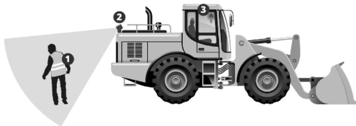
Figure 3: The setup of the case of IR cameras on heavy machines
